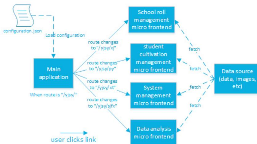
Fig. 9 The application interaction of graduate information system
