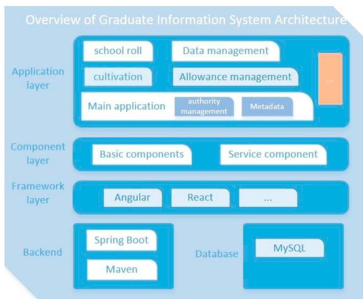
Fig. 7 Overview of Graduate Information System Architecture
